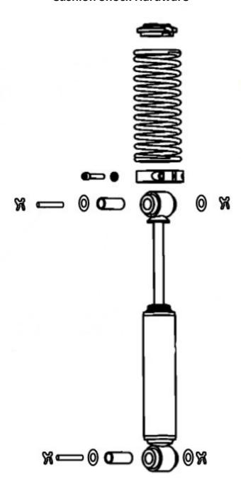
For many years the mounting pins for cushion shock assemblies have used a special pin (000022821), two washers (948975172BG), and two X-washers (936600002BG). This
