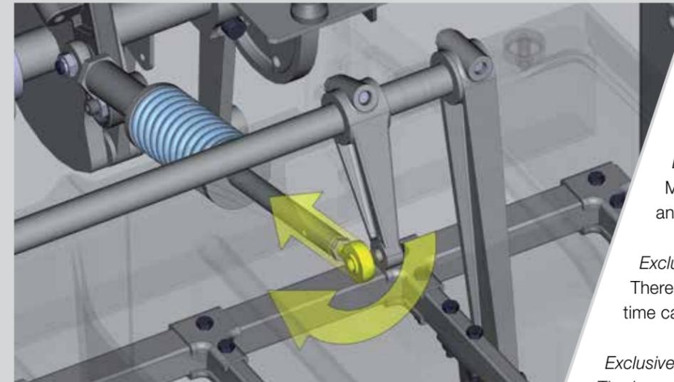
*Sample illustrations from the EDGE Video Training Tool showing the adjustment of the shuttle rod on the pinspotter.*
