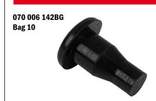
Used to cushion moving parts all over the Distributor, this small bumper can also be found in the PBL Ratchet Crank, behind the Bin Switch Lever, and under the Spotting Solenoid on 82/70's. Washer 948 767 132BG can be sandwiched under the bumper head to adjust the stopping position of moving parts if necessary.
