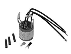
The length of time that the start winding is engaged can be adjusted with this type of solid state start switch. Often known as the "Lewus" switch, this is not recommended for combination motors.
