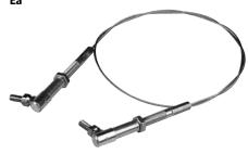
As pins push down the trip arms when they're leaving the distributor, this cable trips the rocker arm and begins the index to the next location. A direct replacement for the old trip rod 070 007 305.
