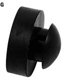
Most commonly used for protecting pins in the Bin assembly, this bumper is also for the start switch lever, and for closed pinwheels on early 82/30's. Made of 100% neoprene rubber for best performance. File off any sharp metal edges around mounting holes prior to installing. Twist them as you press them into place. Some mechanics use a drop of liquid dishsoap on the round surface to help ease installation.
