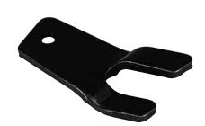
Bolted to the Trip Casting, this part engages the clutch to index the distributor when tripped. If these are binding, the contact surfaces may need to be greased, or may have changed shape from wear.
