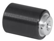
Two of these wheels protrude from the bottom of the lane machine to move it up and down the lane with mimimal effect on the lane conditioning pattern. Replacing old A0994 and A0995 wheels, these are bidirectional and handle heavy oil conditions better than older versions.
