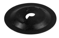
This is the constantly rotating part of the Clutch. Adjusting spring rotation determines it's pressure against the friction disc. To ensure proper operation, the friction surface on this plate must be completely flat, and the opening must screw neatly onto the worm. You can check these by looking for air gaps when you set the plate on a flat surface and when you stack it with another plate.
