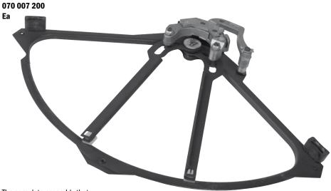
The complete assembly that picks up each standing pin while fallen pins are swept away. Used for pins #1-6 and 8-10. The #7 cell is different from the rest, and there are two different versions of the #7 cell. Early 82/70's with long carb link use #7 Cell 070 007 199. Most have a bolt
