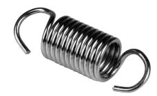
In machines that don't use electronic triggering, this spring holds the lever against the start switch at the top of the cushion shock. Our new improved design prevents end hooks from breaking. Early 82/30's use longer spring 000 021 334.
