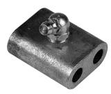
This is what pivots between the two halves of the Front Roller assembly. When assembling, make sure grease zerk points toward the hole in roller body. Interested in trying the lube-free plastic version? If so, order 000 024 760. Always replace these in pairs.
