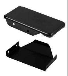
These are located throughout the Bin Assembly and locate each pin as it falls in from the Distributor. When replacing, hold the mounting face of Shock Mount 070 006 354BG tight against the butt guide as you tighten the screws.
