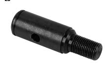
If a front roller pivot stud is worn out, break it out of the kickback plate with a large wrench and replace it with this. File/grind/chisel old weld as necessary to position new stud perpendicular to plate, then secure tightly with 844 074 002BG Nut and 941072200BG washer.
