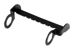
At the bottom of the Distributor Belt's "S" curve, this bracket tensions the belt and helps it track properly. Keep your brackets aligned and seated properly around Tube Assembly 070 006 105.
