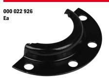
Direct replacement if the Rear Roller Bearing Support breaks on the ball door side. Remove old part, drill holes if necessary and secure with 810 258 100BG screws and 844 058 002BG nuts.
