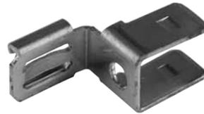
Where two wires connect on the same terminal, this is typically used to accommodate them. In tight locations such as the A&MC Box, bend terminals slightly if necessary so that there is room between neighboring terminals to prevent shorting.
