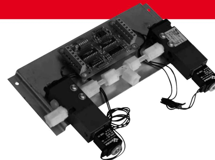
Mounted on the curtain wall, this controls the bumpers on a pair of lanes. For use with scoring system control or front desk switch box. Contains P.C. Board 049 007 125 and Valves 049 007 123.
