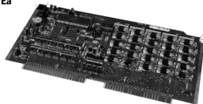
This board puts the microprocessor in the MicroProcessor Chassis. Processes the inputs and determines the outputs to control a 82/70. A direct replacement for all MP boards. Has diagnostic LED's and programmable options.
