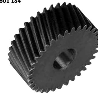
Alternately called "helical gear," it is part of the system that reduces output shaft speed and increases operating torque. When there is breakage or excessive wear, it is best to replace these in sets of three, along with the Ring Gear 785 501 179 and Wheel Shaft 785 501 291.
