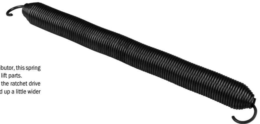
Originally used on the 82/30 distributor, this spring is more often associated with ball lift parts. When using this spring to tension the ratchet drive belt, one hook needs to be opened up a little wider than the original size.
