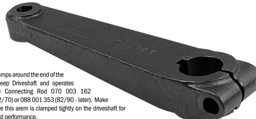
Clamps around the end of the Sweep Driveshaft and operates the Connecting Rod 070 003 162 (82/70) or 088 001 353 (82/90 - later). Make sure this arm is clamped tightly on the driveshaft for best performance.
