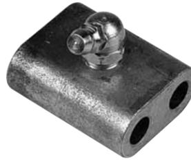
This is what pivots between the two halves of the Front Roller assembly. When assembling, make sure grease zerk points toward the hole in roller body. Interested in trying the lube-free plastic version? If so, order 000 024 760. Always replace these in pairs.
