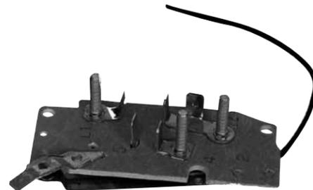
These two switches inside the top of Westinghouse Sweep & Table motors work together to engage the start windings of the motor. The 50Hz Centrifugal Mechanism is still available as part number 785 501 531. The 60Hz mechanism is no longer available, we recommend our Solid State Start Switch 610 309 044 as the best replacement.
