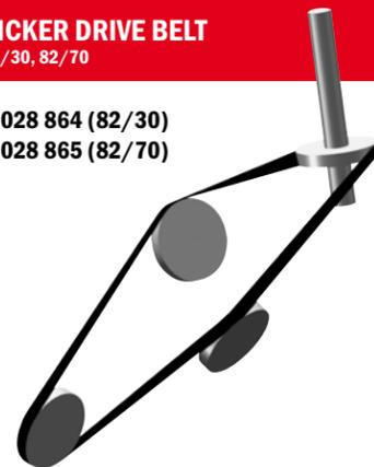
This is the belt that turns the kicker rollers. The 82/30 belt is slightly longer than the 82/70 version.
