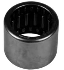
The key to either machine on a pair being able to run the shared ball lift, this clutch bearing locks when turned one direction, and freewheels in the other. This is the same bearing used on the lower shaft of AMF-type front ball returns including C-90, Options and Profile.
