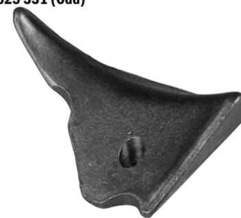
Seven required per pinspotter to hold pins in the pin elevator. If pins are sticking in the wheel and going past the distributor, clean the wheel surface and check these for wear.
