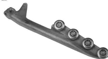
As pins fall off the end of the distributor, they push down these arms and advance the distributor to its next position. Bearings that are missing or that don't spin freely should be replaced with Bearing 000 026 251BG, Screw 813 540 082BG, and Lockwasher 957 100 002BG.
