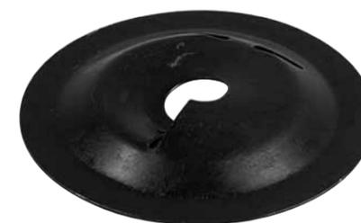
This is the constantly rotating part of the Clutch. Adjusting spring rotation determines its pressure against the friction disc. To ensure proper operation, the friction surface on this plate must be completely flat, and the opening must screw neatly onto the worm. You can check these by looking for air gaps when you set the plate on a flat surface and when you stack it with another plate.
