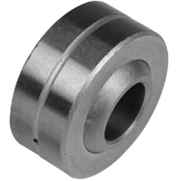
On aluminum tables, this replaces the bearing in the bottom of all 4 yoke legs. Steel tables use different legs, 090 005 545 in front and 090 005 548 in back.
