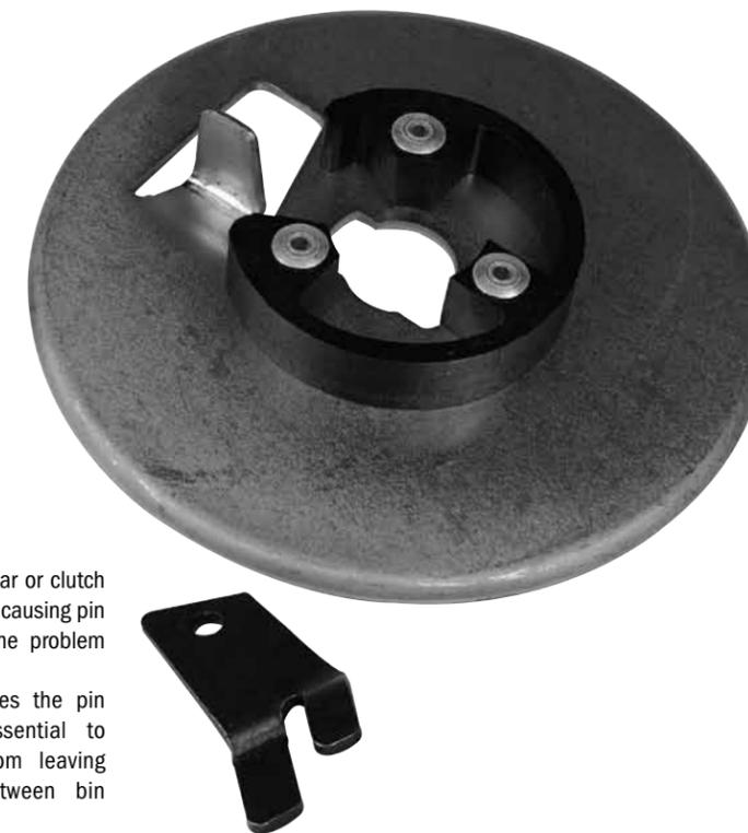
When stop blade wear or clutch plate - pinion slop is causing pin pileups, eliminate the problem with this kit. Clutch plate includes the pin separator ring, essential to preventing pins from leaving the distributor between bin positions. If the stop blades are dragging on this ring, your carriage tubes may be bent.
