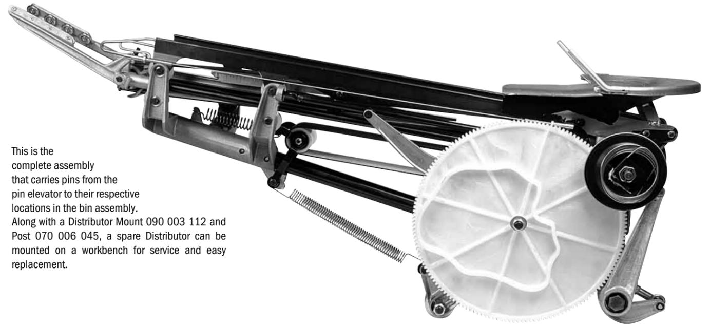
This is the complete assembly that carries pins from the pin elevator to their respective locations in the bin assembly. Along with a Distributor Mount 090 003 112 and Post 070 006 045, a spare Distributor can be mounted on a workbench for service and easy replacement.
