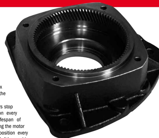
This one-piece ring gear & flange is the part of the gearbox that is mounted to the machine frame. The three planet gears stop in the same location every time. Extend the lifespan of these parts by cranking the motor to a new stopping position every time the gearbox is off of the machine.
