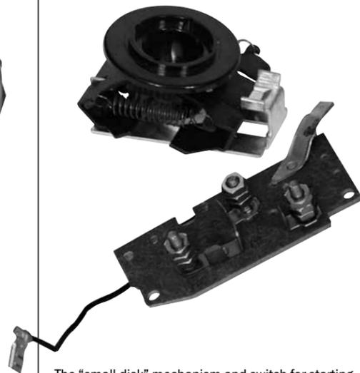
The "small disk" mechanism and switch for starting early model Westinghouse BE motors. If the rotor shaft has worn and no longer supports the mechanism, we recommend replacing it with the 610 309 046 Solid State Switch.
