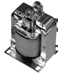
82/30 and early 82/70's use this solenoid to operate parts that determine if the table will pick up standing pins or spot new pins. 30's also use it for pinfeed toggles on their pin elevators. Our solenoids have recently been improved to be more efficient and improve fit and clearance issues.
