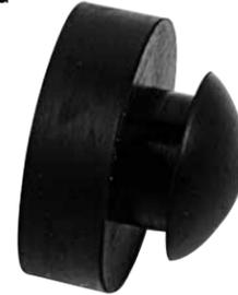
Most commonly used for protecting pins in the Bin assembly, this bumper is also for the start switch lever, and for closed pinwheels on early 82/30's. Made of 100% neoprene rubber for best performance. File off any sharp metal edges around mounting holes prior to installing. Twist them as you press them into place. Some mechanics use a drop of liquid dishsoap on the round surface to help ease installation.
