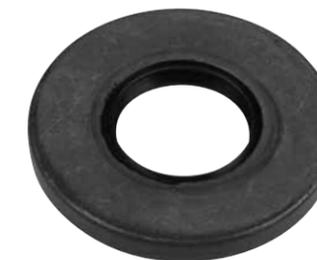
Shaft seals are pressed into gearbox and cap openings to prevent leakage. Prevent future leaks during gearbox rebuilding by dressing off burrs and sharp edges on and around mating surfaces.
