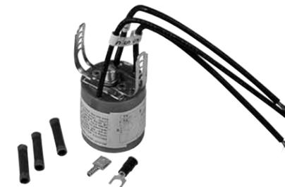
The length of time that the start winding is engaged can be adjusted with this type of solid state start switch. Often known as the "Lewus" switch, this is not recommended for combination motors.
