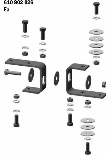
If the back end of a machine migrates away from the front end, it can crack the brackets where the two machine halves meet. Use this kit to repair the damage, and make sure that Floor Bracket 000 026 464 is mounted firmly at both rear corners of the machine.
