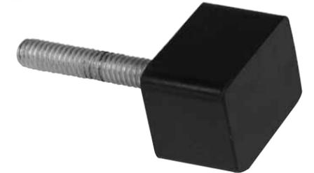
Goes through Sweep Stabilizer (top) Link 070 003 238. During regular inspection, or if your sweep "pops" when it starts down, make sure these are the correct thickness and not sticky. It is a direct replacement for obsolete rubber bumper 000 023 216.
