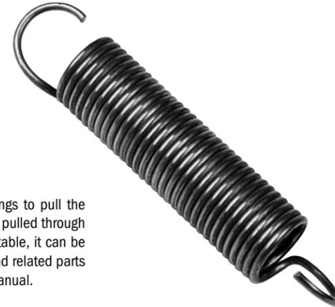
Steel tables use two of these springs to pull the yoke forward. If the spring stud has pulled through the table casting on an aluminum table, it can be replaced by two of these springs and related parts as shown in any steel table parts manual.
