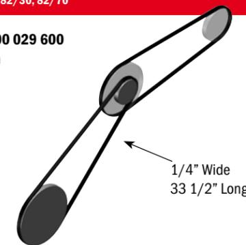
This belt runs between the belt tensioner "mousetrap" pulley and the rudder drive sheave. Measures approximately 33.5" outside.
