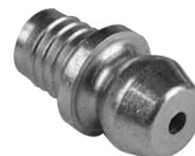
A direct replacement for most grease fittings on various parts of all pinspotters. Self-locking and aligning drivable zerk for 3/16" dia. holes.
