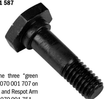
Holds the three "green springs" 070 001 707 on the Spot and Respot Arm Hangers 070 001 751. Always use a new nut 839 665 002BG, and install using Spring Puller Tool 792 505 005.
