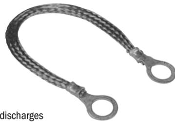
This discharges static electricity that would otherwise build up in the bounce plate assembly. If your scoring system freezes or locks up, inspect to make sure this strap is present, intact, and connected properly.
