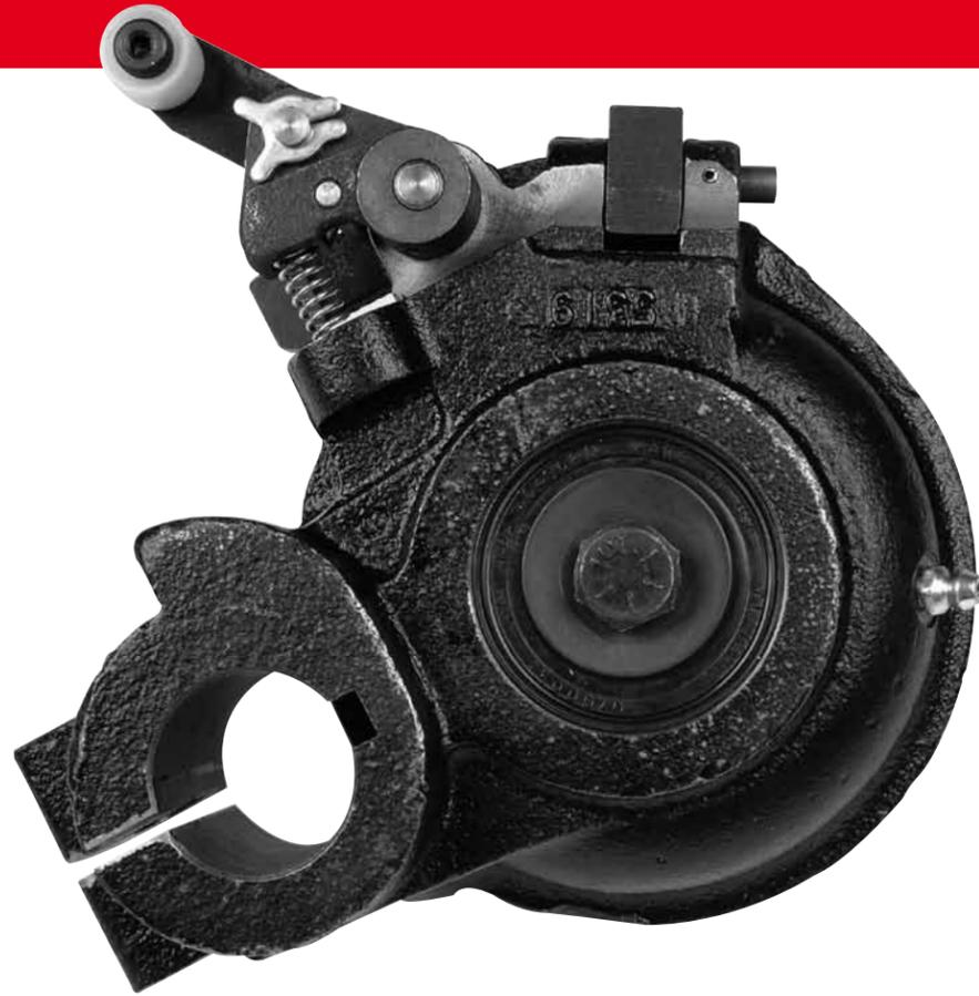
Mounted at the end of the table driveshaft, this controls whether the table lowers to respotting height or to spotting height.
