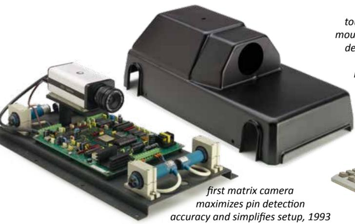
first matrix camera maximizes pin detection accuracy and simplifies setup, 1993
